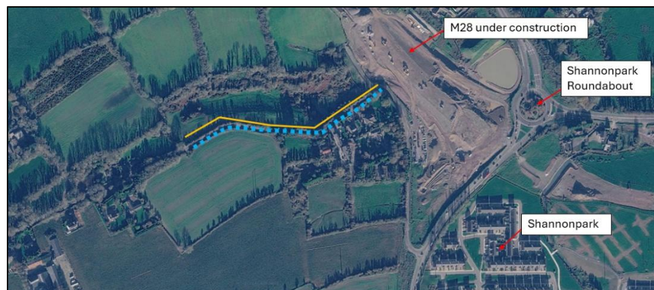
Figure 3.1: Site Context Map showing the approximate section of the grid connection amendment (orange) within the surrounding agricultural lands and the permitted grid alignment along the public road corridor (blue).
